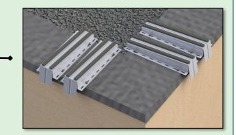
Apply two parallel strips of expanding tape to the top of the retention brackets.
